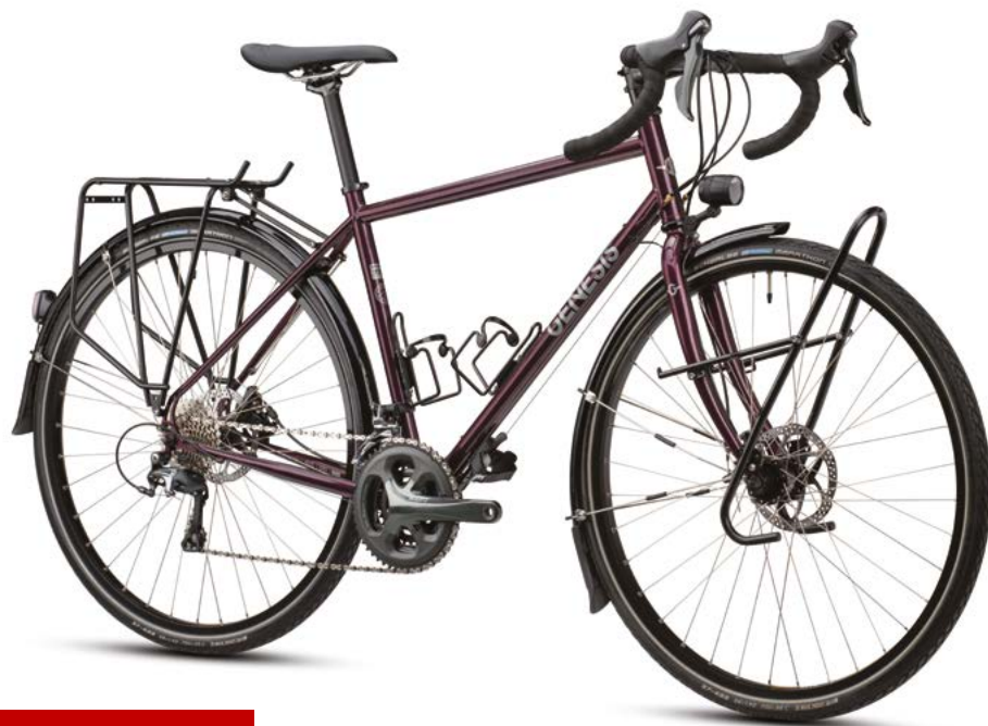
TOUR DE FER 30 Frame: Reynolds 725 Heat-Treated Chromoly Fork: Genesis Full Chromoly Drivetrain: Shimano FC-4703 50/39/30t Brakes: TRP Sphyre-C Rims: Sun Ringle Rhyno Lite, 36h Hubs: Shimano Front - DH-UR700-3D / Rear FH-M6000, 6 Bolt, 36h Tyres: Schwalbe Marathon Weight: 14.73kg Colour: Eagle Eyed Berry Sizes: XS - S - M - L - XL
