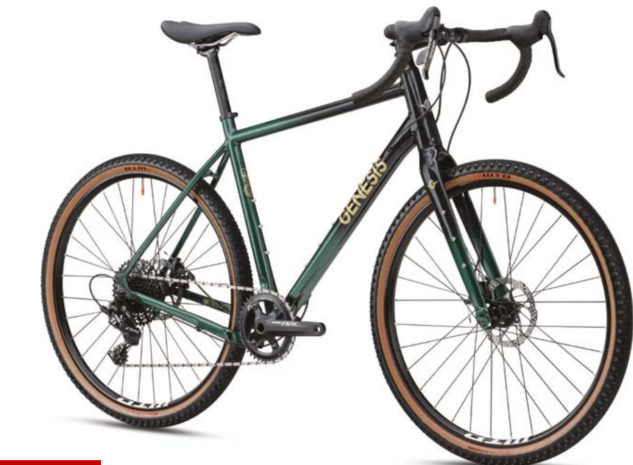
FUGIO 10 Frame: 6061 Aluminium Fork: Genesis Full Carbon Gravel Disc Fork W/ Anything Cage Mounts Drivetrain: SRAM Apex 1 42t Brakes: TRP Spyre-C FM Rims: WTB ST i25 TCS 2.0, 32h Hubs: KT Front - QL-SL2F / Rear QL-X2DR, 6 bolt, 32h Tyres: WTB Venture 650x47c Tubeless Compatible System Weight: 10.5kg Colour: The Black Peas Sizes: XS - S - M - L - XL
