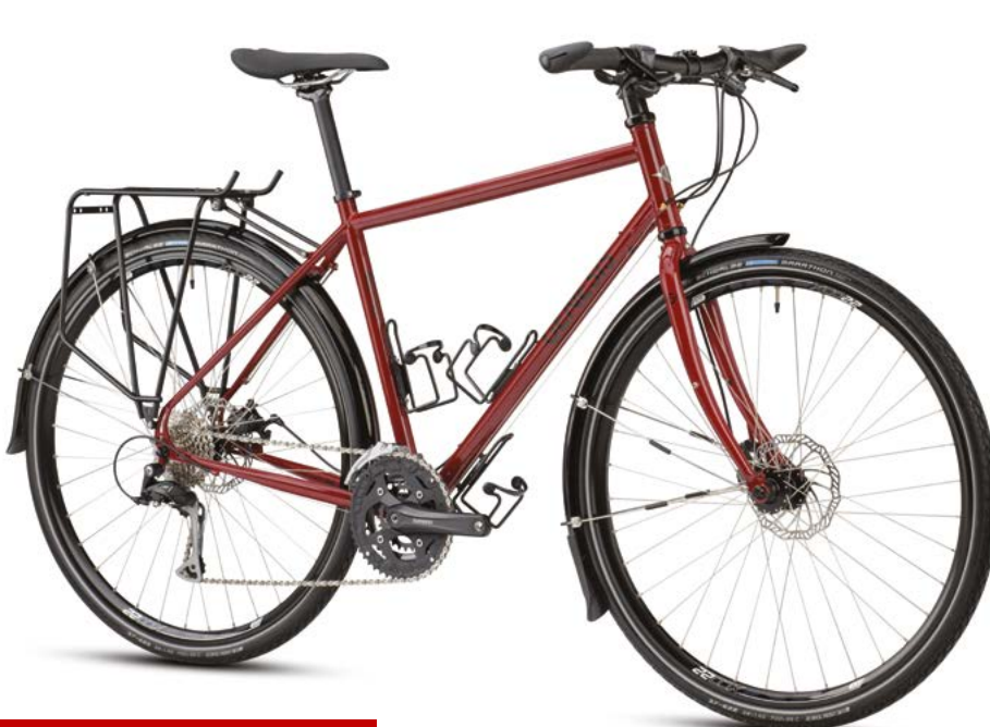
TOUR DE FER 10 FLATBAR Frame: Genesis Mjolnir Seamless Double-Butted Chromoly Fork: Genesis Full Chromoly Drivetrain: Shimano FC-T4010 48/36/26t Brakes: Promax DSK-717RS Rims: Jalco XCD22, 36h Hubs: KT-K08, 6 bolt, 36h Tyres: Schwalbe Marathon Weight: 13.89kg Colour: Red Kennedys Sizes: XS - S - M - L - XL
