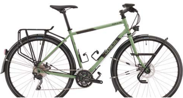
Tour De Fer 20 - Flatbar Frame: Reynolds 725 Heat-Treated Chromoly Fork: Cr-Mo Unicrown Disc Drivetrain: Shimano Deore M610, 44/32/24, 11/32 Wheels: Sun Ringle Rhyno Lite/ 36h, SPPD-8/ Shimano FH-M615 36h/ front/ rear/ 6-bolt/ centre lock Tyres: Schwalbe Marathon Mondial 700x35c Brakes: Promax DSK-717 disc Brakes w/ 160mm Rotors Weight: 15.08kg (Medium w/o Pedals) Additional Info: Trekking mudguards/ Tubus Cargo rear rack/ B&M Cyo Premium Plus headlight/ B&M Secula Plus tail light SRP: £1499.99 Sizes: XS - S - M - L - XL Colour: Matt Dean Green
