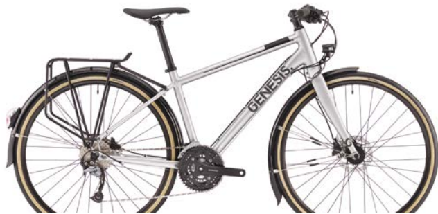
Skyline 30 Frame: ALX8 6066/6061-T6 Double-Butted Aluminium Fork: Genesis Alloy Urban w/ 1-1/8" Alloy Steerer Drivetrain: Shimano Acera, 48/36/26, 11/34 Wheelset: Jalco XCD21/ 32h, Shimano DH-T4051/KT-TC7R 32h/ dynamo front/rear/ centre lock Tyres: CST Sensamo Speed 700x35c 60TPI w/Skinwall Brakes: Shimano BR-M315/ SM-RT10 160mm Rotors Weight: 13kg (Medium w/o Pedals) SRP: £899.99 Sizes: XS - S - M - L - XL Colour: Vivi Silver
