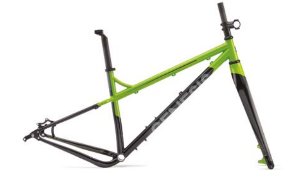
Tarn Frameset Frame: Genesis Mjölínir Seamless Double-Butted Cromoly Fork: Full Carbon 27.5" Fork, Tapered Steerer, 110mm x 15mm Additional Info: Prestine PT-1860/ Bottom Bracket - BSA 73mm Boost (not incl.)/ Front Derailleur - 34.9mm Band-on (not incl.)/ Seatpost - 31.6mm (not incl.) Weight: 3.98kg (Medium Incl. F & R axles, seat collar and headset) SRP: £599.99 Sizes: S - M - L - XL Colour: GTF Green
