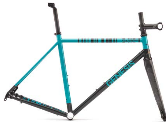
Volare 853 Disc Frameset Frame: Reynolds 853 Seamless Air-Hardening Heat Treated Steel Fork: ADK Full Carbon Road Race Disc w/ 1-1/2" - 1-1/8" Tapered Steerer w/ 12mm TA Weight: 2.82kg (Medium incl. F & R axle, seat collar and headset) Additional Info: Headset - Prestine F-17-A 1-1/8" - 1-1/2" tapered/ BB - Press-fit BB86 (not incl.)/ Front Derailleur - 31.8 Band-on (not incl.)/ Seatpost - 27.2mm (not incl.) SRP: £1199.99 Sizes: XS - S - M - L - XL Colour: Pompey Grey
