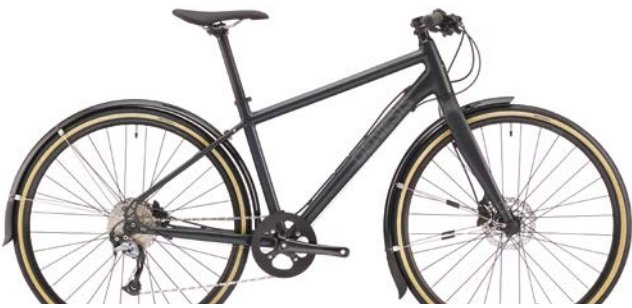
Skyline 10 Frame: ALX8 6066/6061-T6 Double-Butted Aluminium Fork: Genesis Alloy Urban w/ 1-1/8" Alloy Steerer Drivetrain: Shimano Altus/ Acera, Samox 42T, 12/36 Wheelset: Jalco XCD22/ 32h, KT TC7F/TC7R 32h/ front/ rear/ centre lock Tyres: CST Sensamo Speed 700x35c 60TPI w/Skinwall Brakes: Shimano BR-M315 / SM-RT10 160mm Rotors Weight: 11.86kg (Medium w/o Pedals) SRP: £699.99 Sizes: XS - S - M - L - XL Colour: Goodwin's Black
