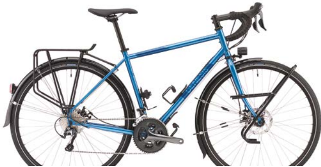
Tour De Fer 30 Frame: Reynolds 725 Heat-Treated Chromoly Fork: Cr-Mo Unicrown Disc Drivetrain: Shimano Tiagra 4703, 50/39/30, 11/32 Wheels: Sun Ringle Rhyno Lite/ 36h, SP PD-8/ Shimano FH-M615 36h/ front/ rear/ 6-bolt/ centre lock Tyres: Schwalbe Marathon Mondial 700x35c Brakes: TRP Spyre-C 2-piston Mechanical disc brake w/ 160mm TR160 Rotors w/ rear adapter Weight: 15.86kg (Medium w/o Pedals) Additional Info: Trekking mudguards/ Tubus Cargo rear rack/ Tubus Tara front rack/ B&M Lumotec IQ-X headlight/ B&M Secula Plus tail light SRP: £1799.99 Sizes: XS - S - M - L - XL Colour: Dibden Blue
