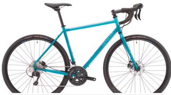
Croix De Fer 30 Frame: Reynolds 725 Heat-Treated Chromoly Fork: Cr-Mo Unicrown Disc Drivetrain: Shimano 105 5800 Wheels: Jalco SR240D/ 32h, Shimano RS-505 32h/ front/ rear/ centre lock Tyres: Clement X'Pior USH 700x35c 60TPI Brakes: Shimano BR-RS505 hydraulic Brakes w/ Shimano SM-RT54 160mm Rotors Weight: 11.58kg (Medium w/o Pedals) SRP: £1799.99 Sizes: XS - S - M - L - XL Colour: Hawkins Green
