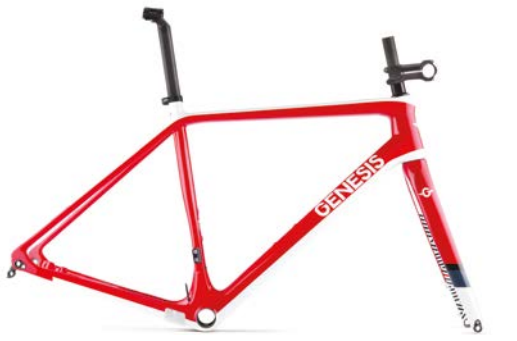
Vapour Carbon CX Team Frameset Frame: 30/40T Modulus Carbon CX w/ Tapered Headtube & Fully Internal Cable Routing Fork: Genesis Carbon CX w/ 1-1/2" - 1-1/8" Tapered Steerer w/ 12mm Thru-Axle Weight: 1.72kg (Medium incl. F & R axle, seat collar and headset) Additional Info: Headset - Prestine PT-1860A sealed 1-1/8 ACB Top, 1-1/2" industrial sealed / BB - B86 Press-fit (not incl.) / Front Derailleur - Braze-on (not incl.) / Seatpost - 27.2mm (not incl.) SRP: £1499.99 Sizes: XS - S - M - L - XL Colour: Smash Red
