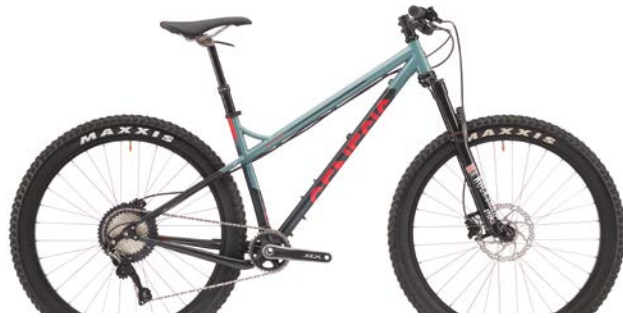
Tarn 20 Frame: Genesis Mjölínir Seamless Double-Butted Cromoly Fork: Rockshox Pike RL, Solo Air, 120mm, Tapered Steerer, 110mm x 15mm Drivetrain: Shimano SLX 1 x 11 speed Wheels: WTB Scraper 40mm Tubeless-Ready, 32h Tyres: Maxxis Rekon 27.5x2.8" Brakes: Shimano MT500 180/160mm Weight: 13.96kg (Medium w/o Pedals) SRP: £1999.99 Sizes: S - M - L - XL Colour: Red Dave's Slate
