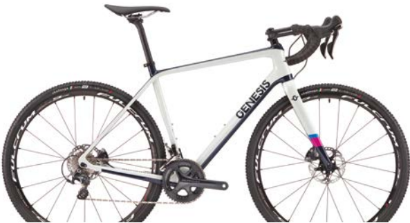
Vapour Carbon CX 30 Frame: 30/40T Modulus Carbon CX w/ Tapered Headtube & Fully Internal Cable Routing Fork: Genesis Carbon CX w/ 1-1/2" - 1-1/8" Tapered Steerer w/ 12mm Thru-Axle Drivetrain: Shimano Ultegra 6800 Wheelset: Fulcrum Racing 5DB Tyres: Challenge Grifo CL 700x33c 60TPI Brakes: Shimano BR-RS805 hydraulic Brakes w/Shimano SMRT81 160mm Rotors Weight: 8.60kg (Medium w/o Pedals) 1.72kg (Frameset) Complete Bike: SRP: £2999.99 Sizes: XS - S - M - L - XL Colour: Devonport Grey Frameset: SRP: £2799.99 Sizes: XS - S - M - L - XL Colour: Devonport Grey
