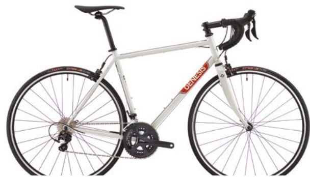
Equilibrium 20 Frame: Reynolds 725 Heat-Treated Chromoly Fork: Carbon Road w/ 1-1/8" Alloy Steerer Drivetrain: Shimano 105 5800 Wheels: Jalco DRX20/ 28h, KT-G15F/G1ER 28h/ front/ rear Tyres: Clement Strada LGG 700x25c 60TPI Brakes: Promax RC-482 Weight: 9.44kg (Medium w/o Pedals) SRP: £1399.99 Sizes: XS - S - M - L - XL Colour: Mainey Grey
