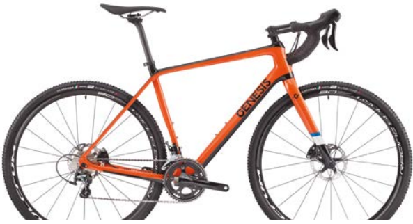
Vapour Carbon CX 10 Frame: 30/40T Modulus Carbon CX w/ Tapered Headtube & Fully Internal Cable Routing Fork: Genesis Carbon CX w/ 1-1/2" - 1-1/8" Tapered Steerer w/ 12mm Thru-Axle Drivetrain: Shimano Tiagra 4700 Wheelset: Fulcrum Racing Sport DB Tyres: Challenge Grifo CL 700x33c 60TPI Brakes: Shimano BR-RS405 hydraulic Brakes w/Shimano SMRT81 160mm Rotors Weight: 9.02kg (Medium w/o Pedals) SRP: £2099.99 Sizes: XS - S - M - L - XL Colour: Traffic Orange
