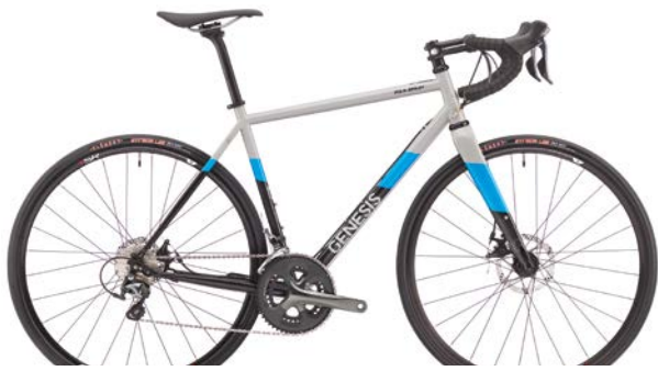
Equilibrium Disc 10 Frame: Genesis Mjölafir Seamless Double-Butted Cromoly Fork: Carbon Road Disc w/ 1-1/8 Drivetrain: Shimano Tiagra 4700 Wheels: Genesis SR220/ 28h, Formula RX812/RX300 28h/ front/ rear/ centre lock Tyres: Clement Strada LGG 700x28c 60TPI Brakes: TRP Spyre-C 2-piston Mechanical disc brake w/160/140mm TR160 Rotors Weight: 10.86kg (Medium w/o Pedals) SRP: £1499.99 Sizes: XS - S - M - L - XL Colour: Gamble Grey
