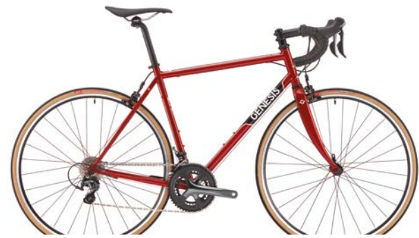
Equilibrium 10 Frame: Genesis Mjölhir Seamless Double-Butted Cromoly Fork: Carbon Road w/ 1-1/8" Alloy Steerer Drivetrain: Shimano Tiagra FC-4700 Wheels: Jalco DRX20/ KT-G15F/G1ER 28h/ front/ rear Tyres: Clement Strada LGG 700x25c 60TPI Brakes: Promax RC-482 Weight: 9.76kg (Medium w/o Pedals) SRP: £999.99 Sizes: XS - S - M - L - XL Colour: Rubv Red
