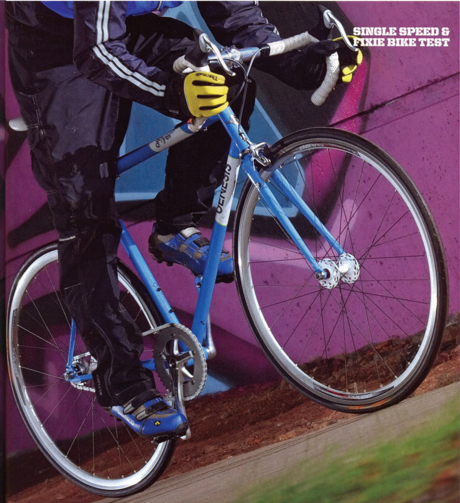
The Genesis uses the same Reynolds 520 double-butted Crommo steel main tube mix as the Dawes for a resilient baseline
