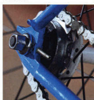
Slim threaded bolts screw in and out on either side to keep the rear wheel correctly aligned
