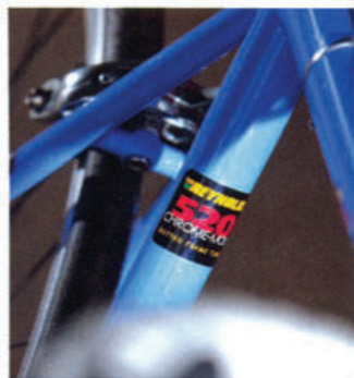
The Genesis uses the same Reynolds 520 double-butted Crommo steel main tube mix as the Dawes for a resilient baseline
