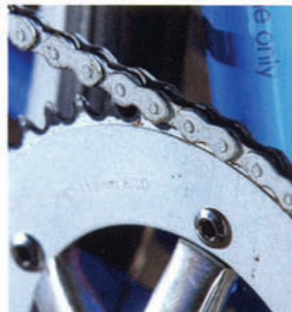
The 46-tooth chainring and short cranks give more cornering clearance in the fixed mode
