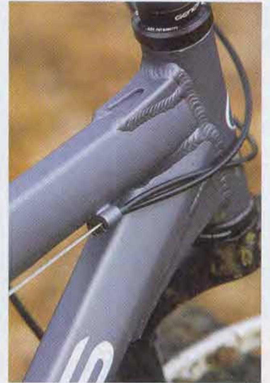
Nice tube profiling and good reinforcing behind the head tube
